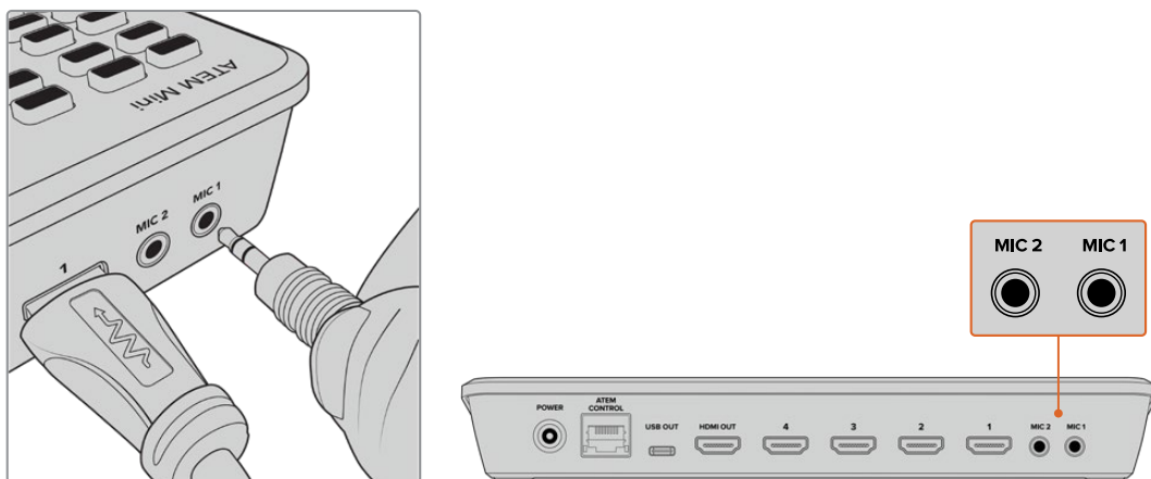
Connect microphones to ATEM Mini's mic inputs
